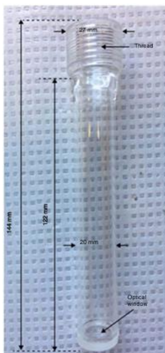
Figure 3: Image showing the size and dimension of ECL cell/cuvette
