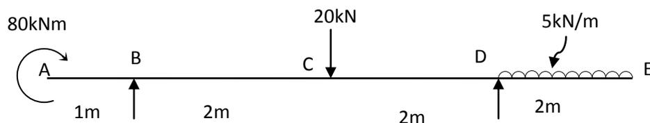
11. Calculate the maximum deflection and maximum slope for the beam shown in fig. below. (20)
