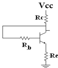
Derive temperature stability factor of the above bias circuit
